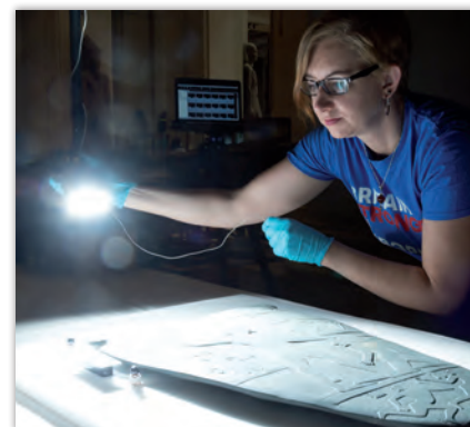
Reflectance Transformation Imaging involves the systematic application light from different positions and angles to the artefact surface. Photograph: Ahmed Amin.
